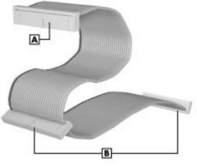
${\bf A}$  – Connects to System Board IDE Port  ${\bf B}$  – Connects to IDE Devices
